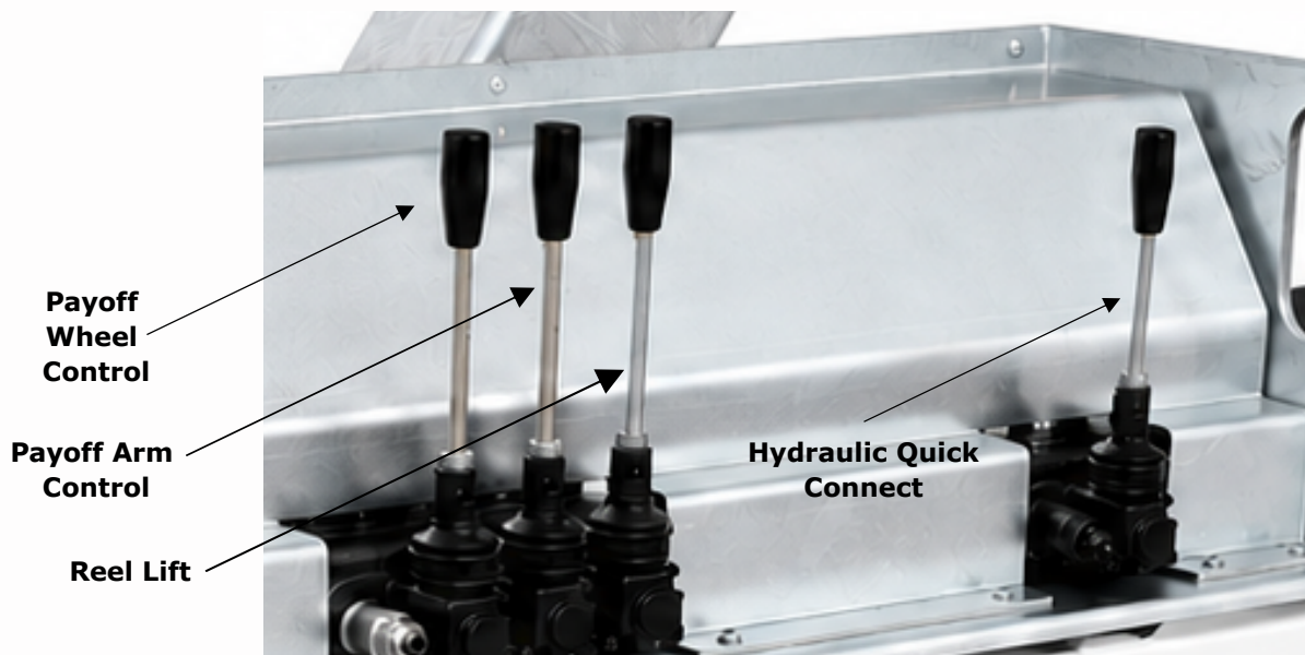
Figure 7: Hydraulic Control Valves
